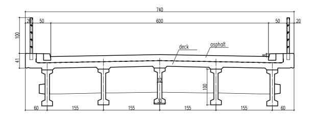
Figure 1. Bridge cross-section.
