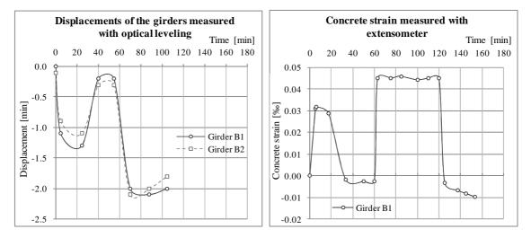
Figure 4. Vertical displacements and concrete strains at the girders' midspan.
