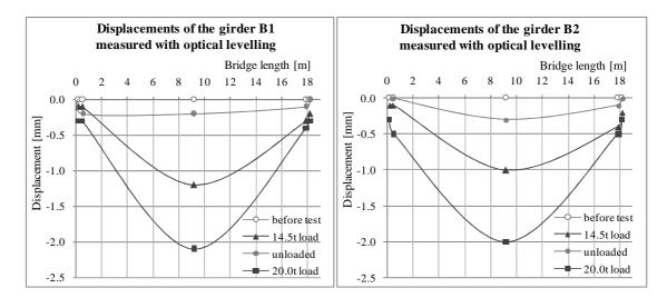
Figure 5. Vertical displacements of the girders at different phases of the test.
