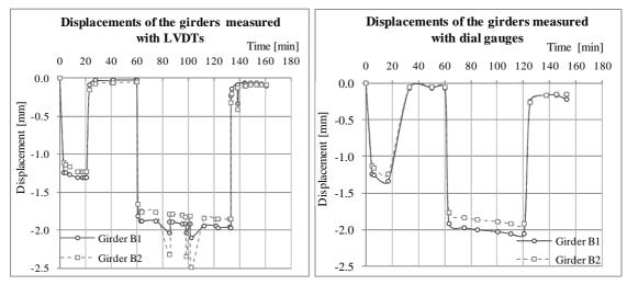
Figure 3. Vertical displacements of the girders' midspan.
