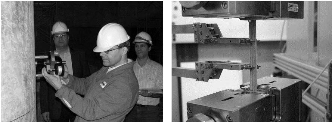
Figure 7: Hotel Parsian Azadi, in situ tests for CFRP installation quality control (Left), laboratory tests at EMPA for material quality assurance (Right)
