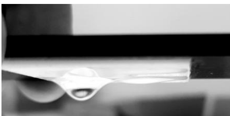
Figure 7. Capillary formation in the housing of the sensor system.
