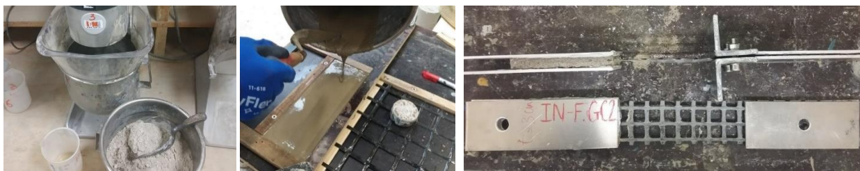
(a) Preparation step of the cementitious matrix (b) Molding the specimen plate (IN-F.GC1) (c) Labeling of the pull-out test specimens (IN-F.GC2)
