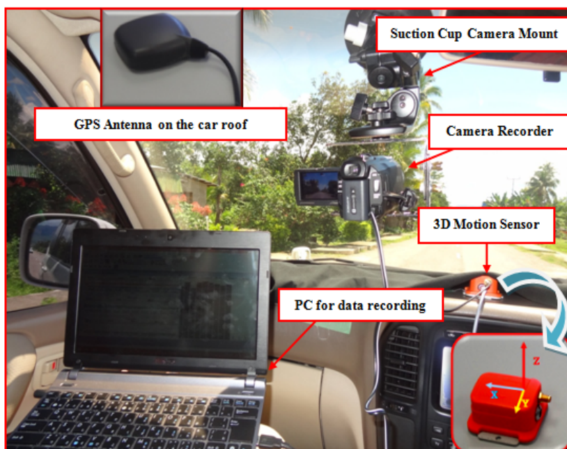
Figure 1. Arrangement of measuring equipment installed in a car.
