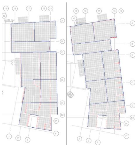
Figure 7. Mode shapes for the first two eigen modes.
