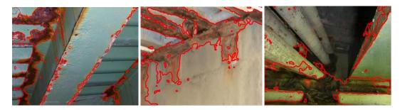
Figure 4. Sample results of corrosion detection and segmentation
