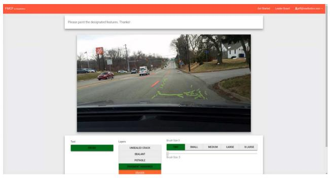
Figure 1. Annotation of distresses by painting over them using custom web-based labeling platform.
