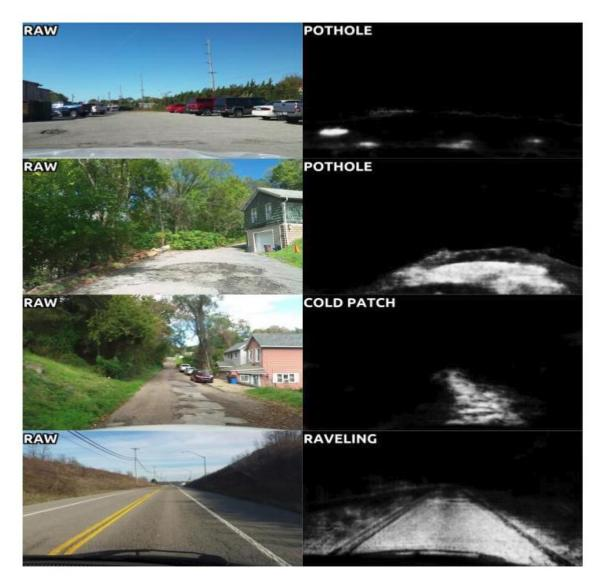
Figure 3. Selected segmentations from our deep learning model. Left column contains raw video frames. Right column contains model output where grayscale value indicates probability (i.e. black = 0%; white=100%).
