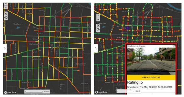
Figure 6. Network level display of ratings. The left image shows ratings that have been averaged on intersection-to-intersection road segments. The right image shows individual images that are sampled every 3 meters along the road. Users can click the points or segments to display additional information, such as to view the associated image.
