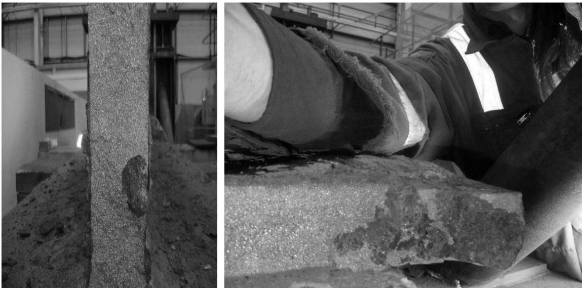
Figure 4. Failure surface of the unreinforced girder, web left, flange right. Note the inclusions.
