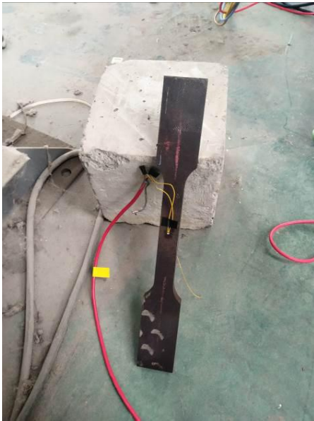
Figure 5. Layout of temperature compensation measuring points
