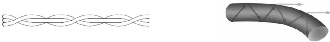
Figure 1. Schematic of braided fiber optics (left) and light flux in the Optical Strand (right)
