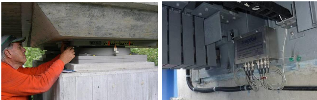
Figure 2. Traditional approach to measurements during inspection visits (left), and continuous automated measurement by means of SHM (right).
