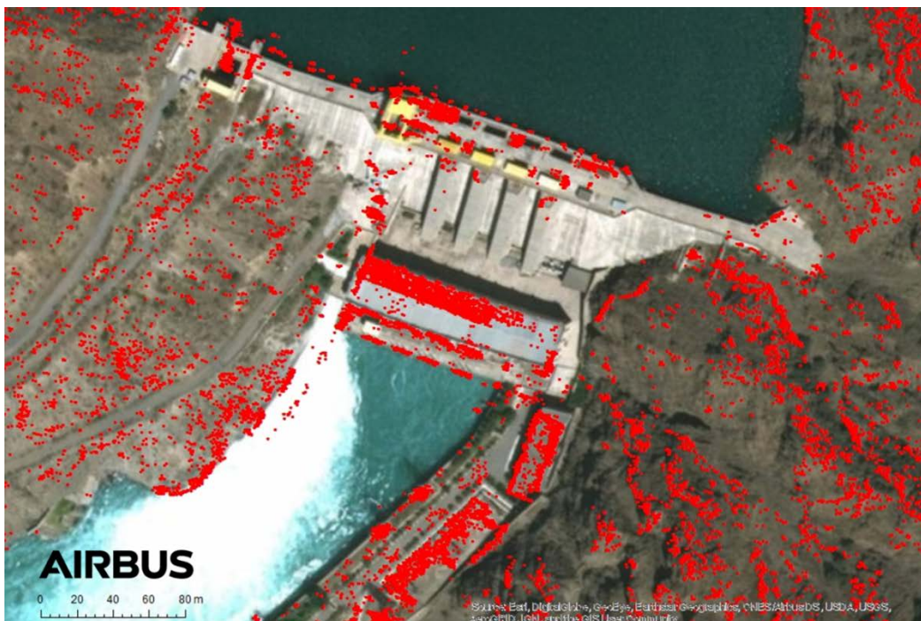
Figure 5. Overview about the location of measurement points (red points) at the dam and its immediate surroundings as result of the descending PSI analysis (© DLR e.V. 2017-2018 and © Airbus Defence and Space GmbH 2019).
