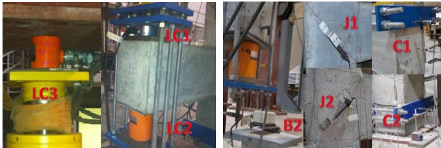
Figure 7. Test specimen with Load cells and LVDT's.
