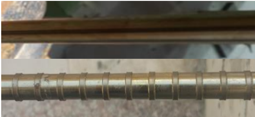
Figure 2. SMA bars before and after ribs creation.
