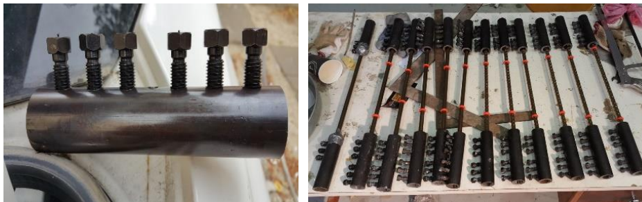
Figure 3. The mechanical coupler with SMA bars for tension testing.
