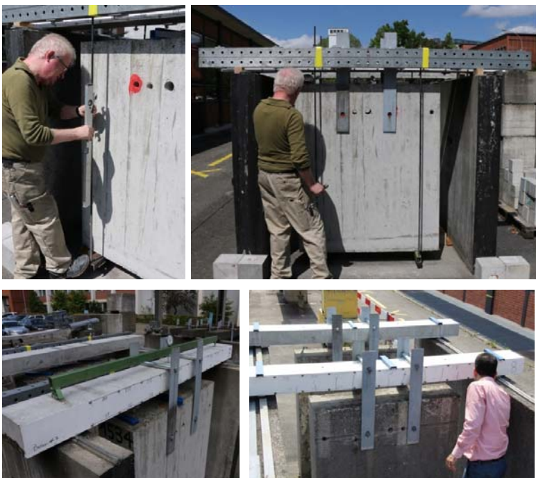
Figure 6: Top: Application of sustained load. Bottom: a photo of the mid-span deflection measurement of activated beam and a photo of the crack propagation marking
