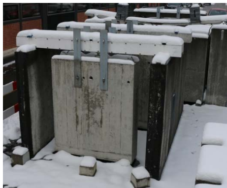
Figure 7: A photo of both beams in winter. Depth of the snow is approximately 80 mm
