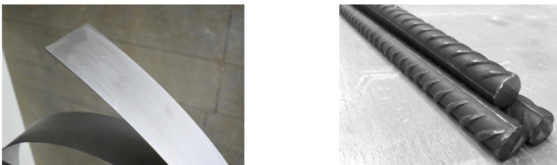
Figure 1. Memory-steel strips ‘re-plate’ (left), Memory-steel bars ‘re-bar’ (right)
