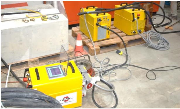
Figure 4: Power supply device to activate ‘memory steel’ stirrups
