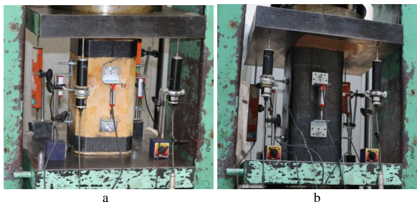
Figure 1. The test setup of a) a reference specimen and b) a confined specimen
