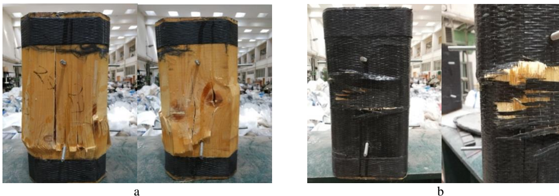
Figure 2. a) Reference specimens and b) S-1-30 and S-1-40 specimens after tests
