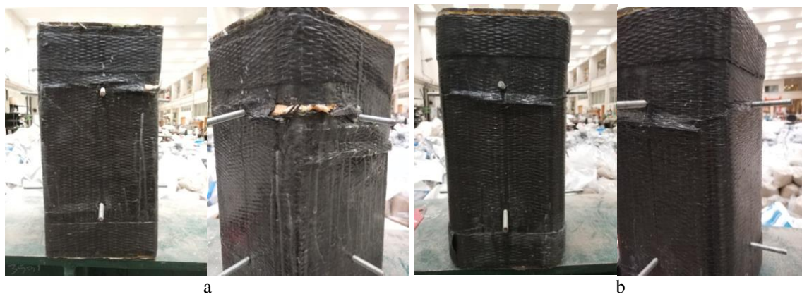
Figure 3. a) S-1-0 series and b) S-3-30 series after tests
