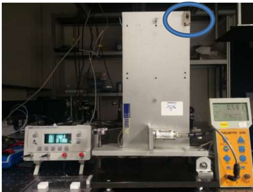
Figure 5. The optical setup for the characterization of the manufactured chips.
