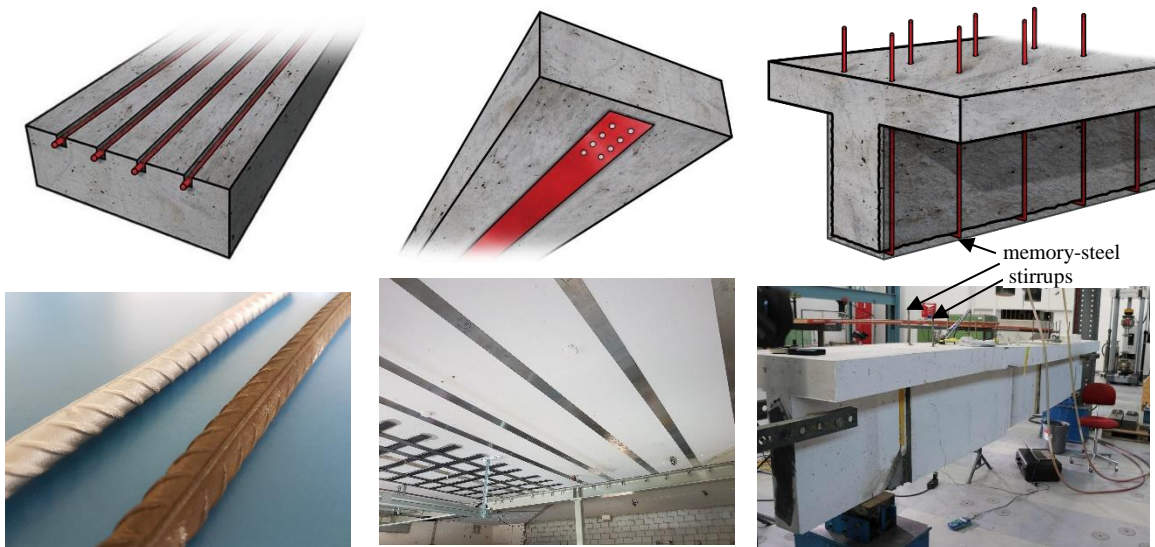
Figure 6. Flexural strengthening of RC beams with memory-steel bars grouted in grooves in the concrete surface (NSMR).
