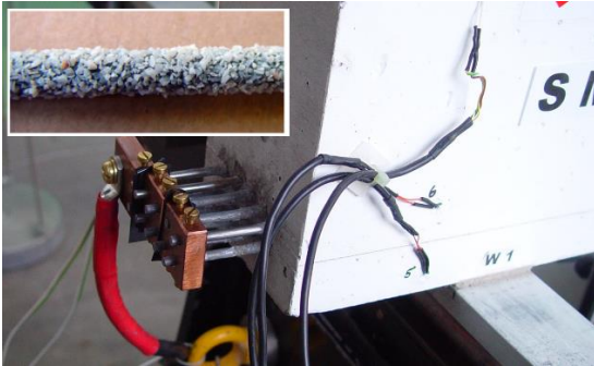
Figure 2: Concrete beam reinforced with NiTi wires, copper clamps for electrical resistive heating, quartz sand treatment (zoom) of the NiTi wires for better bond to the concrete.
