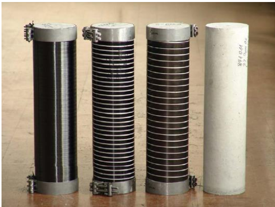
Figure 4: Test specimens to investigate the effect of prestressed confinement, Janke et al. (2009).
