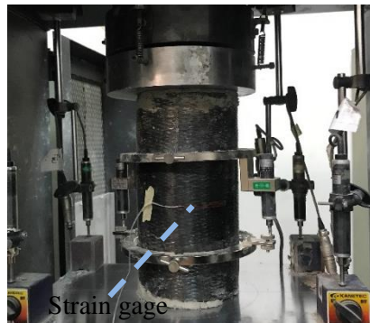
Fig. 2. Test setup for specimens illustrating LVDT and strain gauge application
