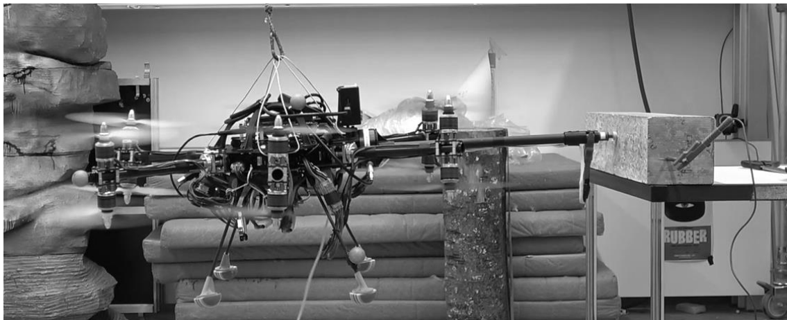
Figure 2. Flying corrosion inspection robot (hexarotor) with inclined propellers measuring electrical concrete resistances and potentials on a concrete block (side A) secured by a safety rope from the top.
