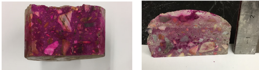
Fig. 4: Carbonation depth test (A) Southview Bridge (B) Sierrita de la Cruz Creek Bridge
