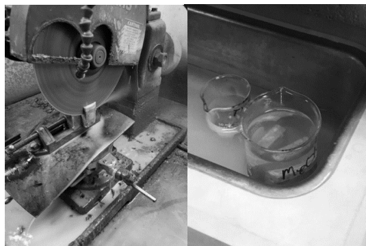
Fig. 1: Specimens preparation (A) SEM and EDS sectioning (B) sonic bath
