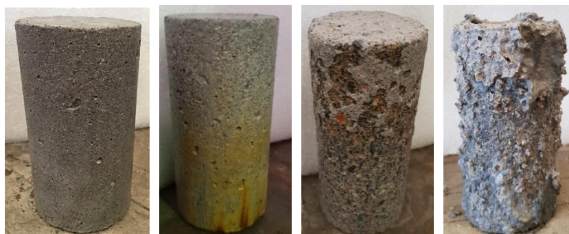
Figure 1. Samples after exposure to sulfuric acid (From left 2, 4, 8 & 12 weeks).
