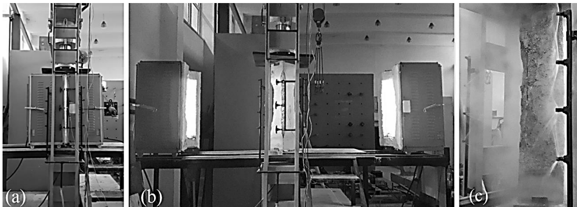
Figure 4. Views from tests: a) Heating b) Just after heating c) Water-cooling.
