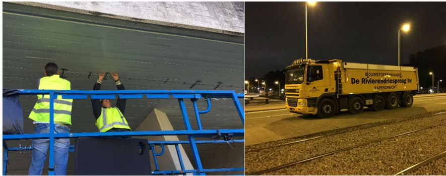
Figure 5. (Left) Gluing the sensing fiber between position A and D. (Right) Using a truck with constant speed to generate a moving load.
